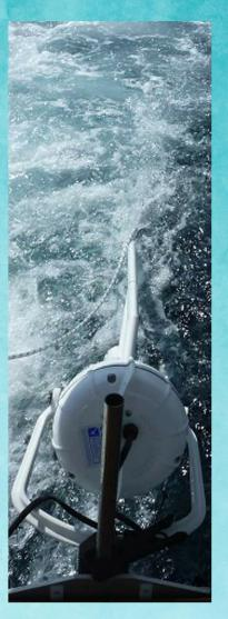
The Sail-Gen generates approximately 230 amp-hours per day at 6 knots, rising to 500 amp-hours at 8 knots.
