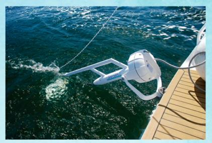
The Sail-Gen Lite comprises a rigid welded aluminium frame with a carbon fibre drive shaft and cast alloy alternator housing and water impeller.
