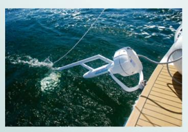
The Sail-Gen comprises a rigid welded aluminium frame with a carbon fibre drive shaft and cast alloy alternator housing and water impeller.
