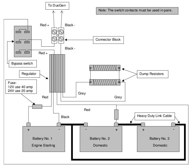
Domestic Batteries 2 & 3 are shown connected in parallel
