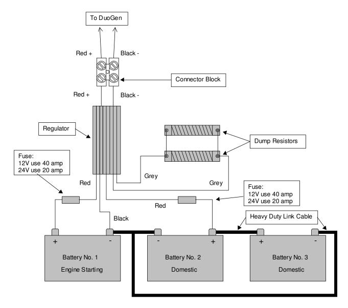
Domestic Batteries 2 & 3 are shown connected in parallel
