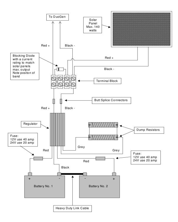
DuoGen Twin Battery Voltage Regulator Wiring Diagram with Three Batteries / Banks
